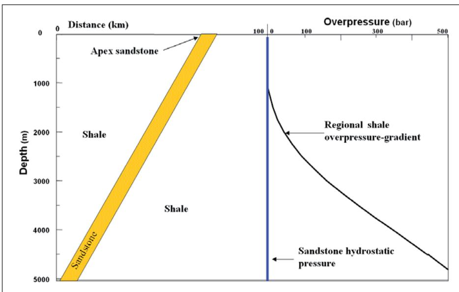
Figure 1. Cross section used to exemplify the pore pressure distribution (right) in a simple sandstone/shale system (left).
