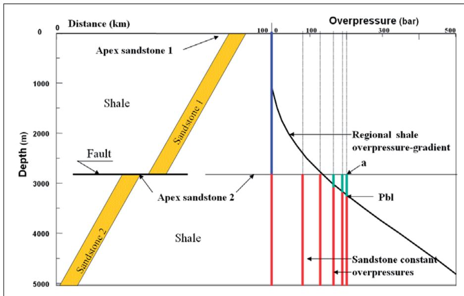
Figure 2. The sandstone in the cross section in Figure 1 has been offset by a horizontal fault (left). The inferred pore pressure development in the system is shown to the right.
