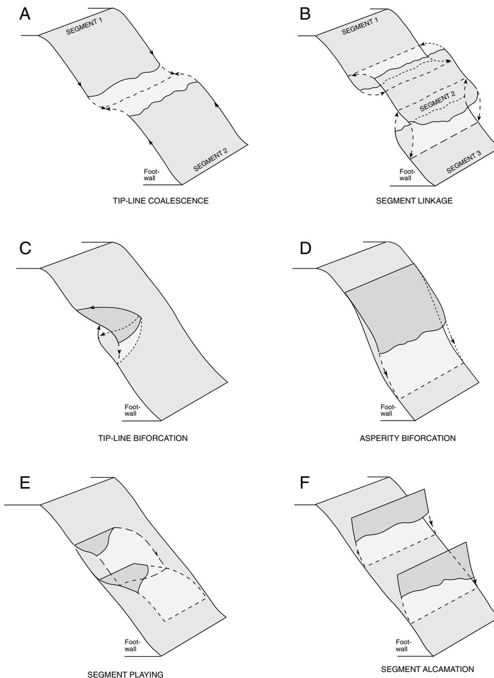
Figure 6. Principal configurations of fault segments during development of fault lenses. (a) Tip-line coalescence, (b) segment linkage, (c) tip-line bifurcation (d) asperity bifurcation, (e) hanging-wall segment splaying, (f) hanging-wall segment amalgamation. The most common mechanisms observed in the present data are segment linkage and asperity bifurcation. Modified from Gabrielsen & Clausen (2001).
