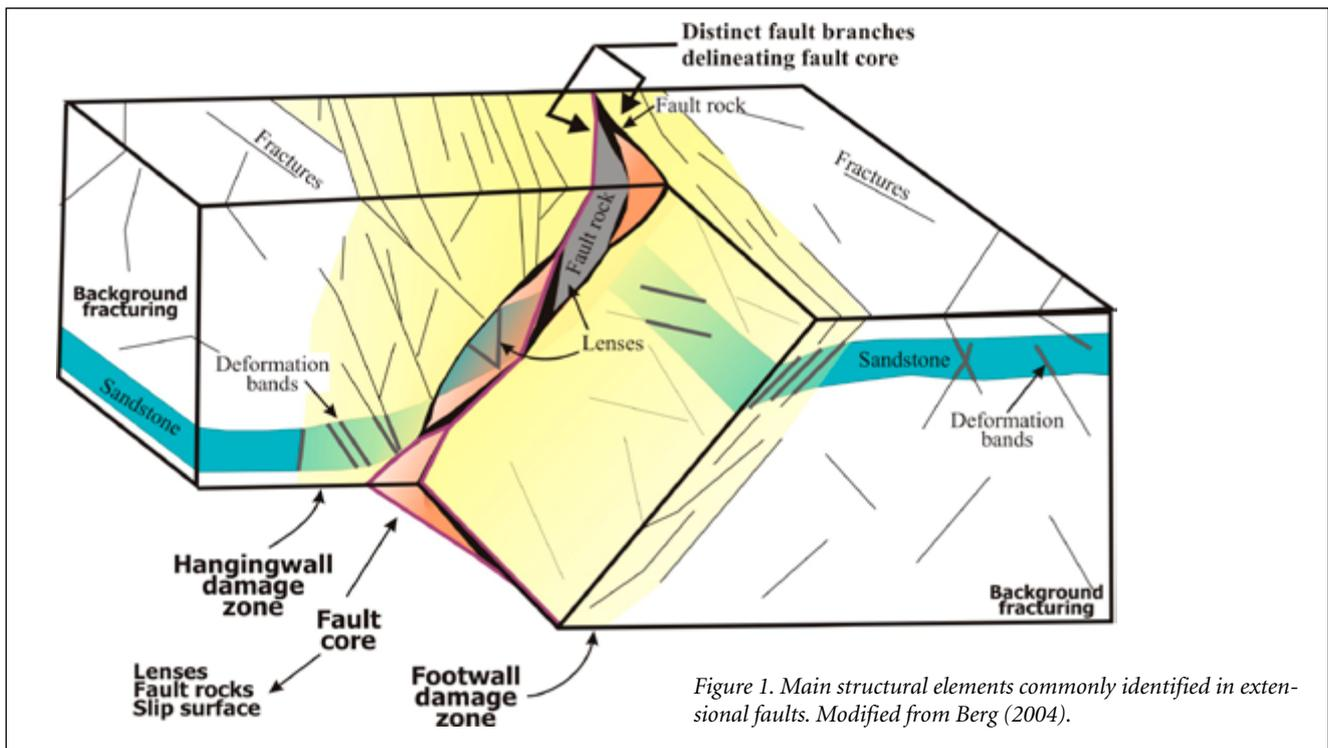
Figure 1. Main structural elements commonly identified in extensional faults. Modified from Berg (2004).
