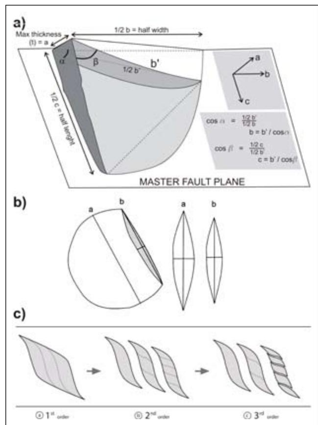
Figure 2. a) Fault lens with kinematic axes and dimensions as measured in the field. Calculation of  $a$ -axis and  $b$ -axis from observed section (shaded in grey) is indicated. b) Because of the symmetry of the lenses, the  $c$ : $a$  ratio (dip:thickness-axes ratio) is robust even in cases where the entire lens is not available for measurement. c) Progressive break-down of lenses produces lenses of different "orders".
