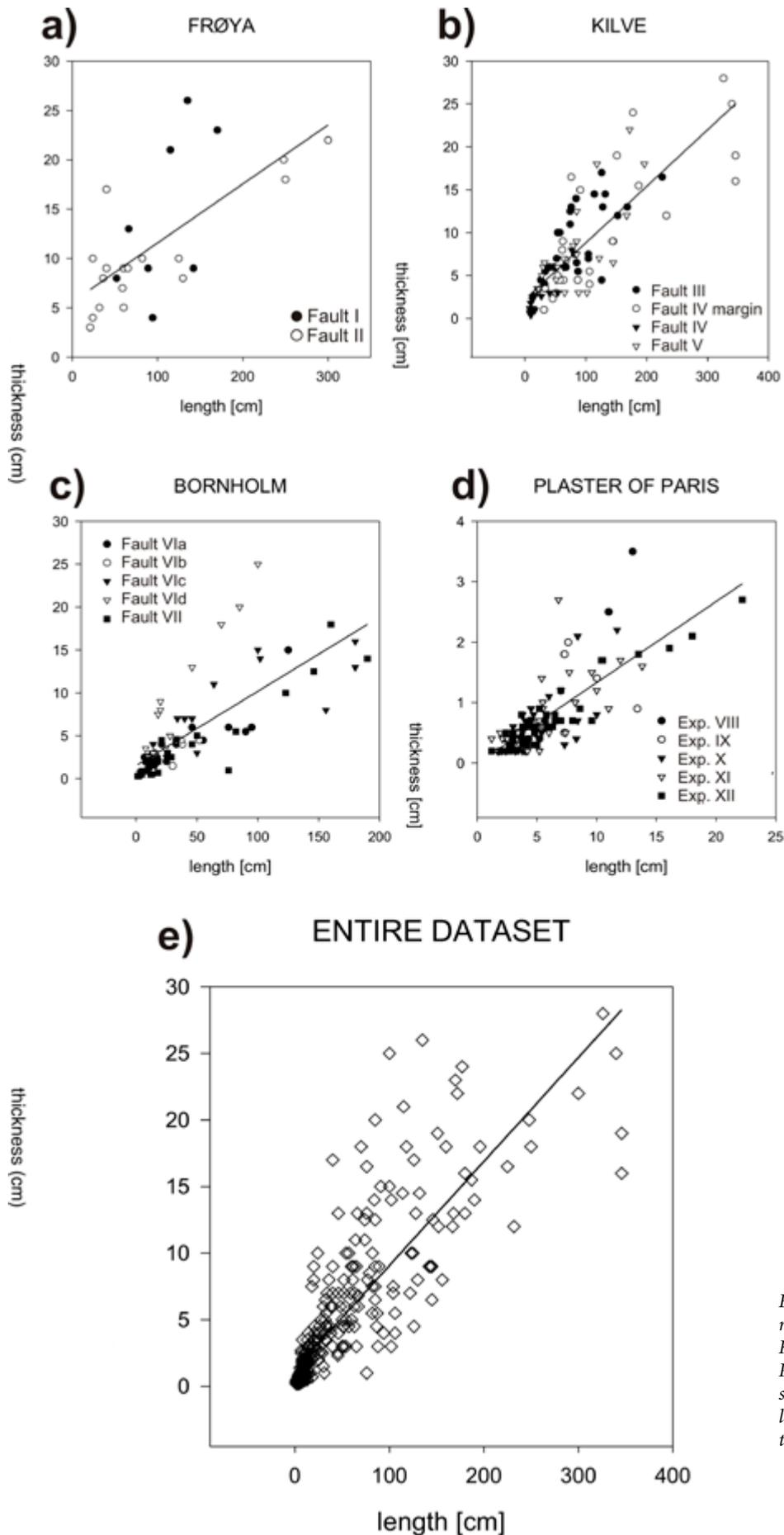
Figure 7. Plot of length versus thickness-ratio (c:a) of the lenses on (a) Frøya, (b) Kılve, (c) Bornholm and (d) plaster-of-Paris analogue experiments. The regression line in each plot represents all the lenses for that specific area. (e) Plot of the complete data set. See also Table 1.
