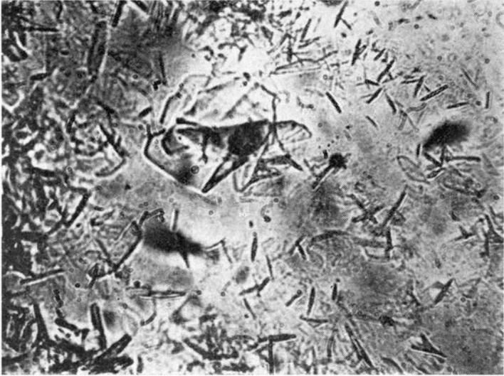
Fig. 2. Normal habit of albite obtained by devitrification above  $1020^{\circ}\text{C}$ .
