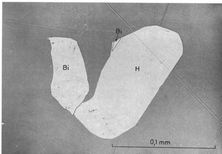
Fig. 2. A composite grain of hedleyite (H) and bismuth (Bi) in galena. Polished section, 1 nicol, oil immersion.
