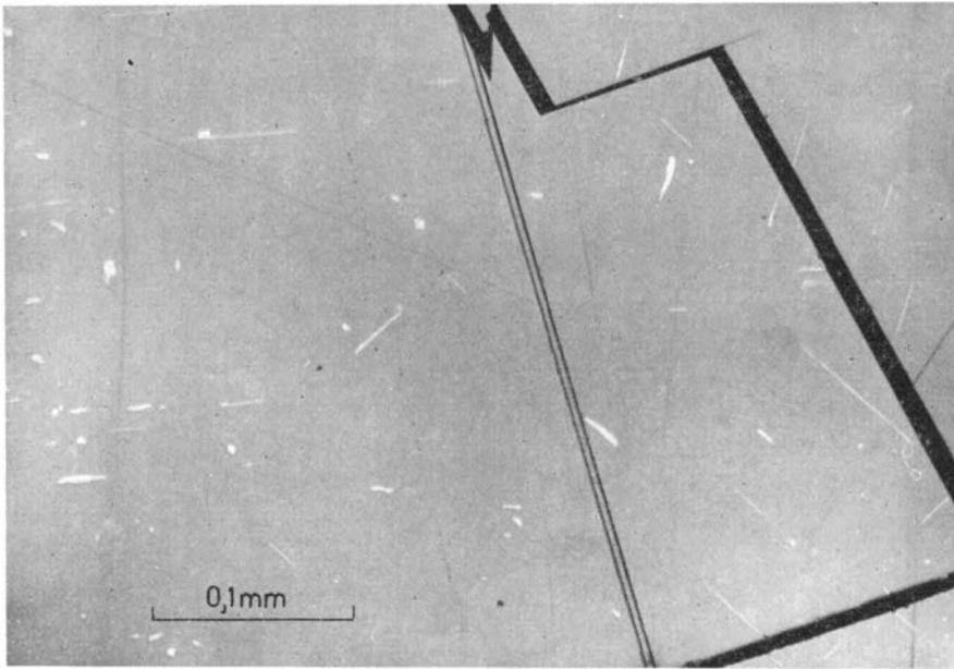
Fig. 3. Thin laths of hedleyite and bismuth (white) crystallographically orientated in galena. The cubic cleavage in the galena can be seen. Polished section, 1 nicol, oil immersion.
