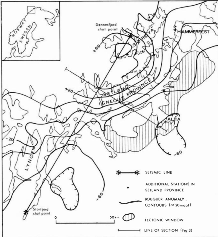
Fig. 1. Location of seismic line in relation to the Bouguer anomaly field and geological provinces.
