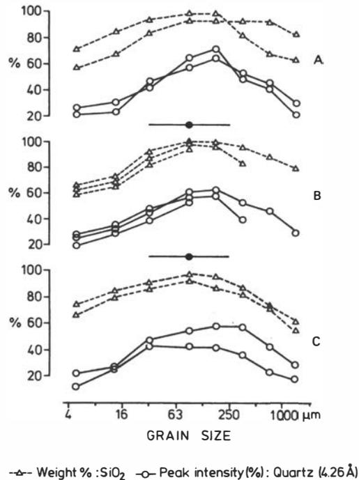
Fig. 8. Plot of the X-ray intensity percentage for quartz and weight % for SiO<sub>2</sub> for the silt and sand fractions for the different facies. (A: Poorly sorted sand, B: Unconsolidated mud, C: Pebbly mud (till ?).
