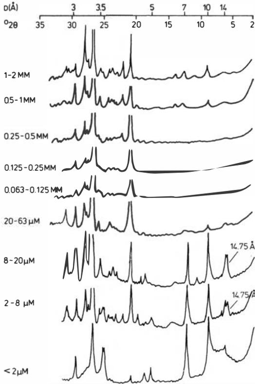
Fig. 5. X-ray diffraction pattern for the sand-silt-clay fractions of Quaternary superficial sediments; North Sea, northeastern part. The samples were saturated with Sr<sup>++</sup>.
