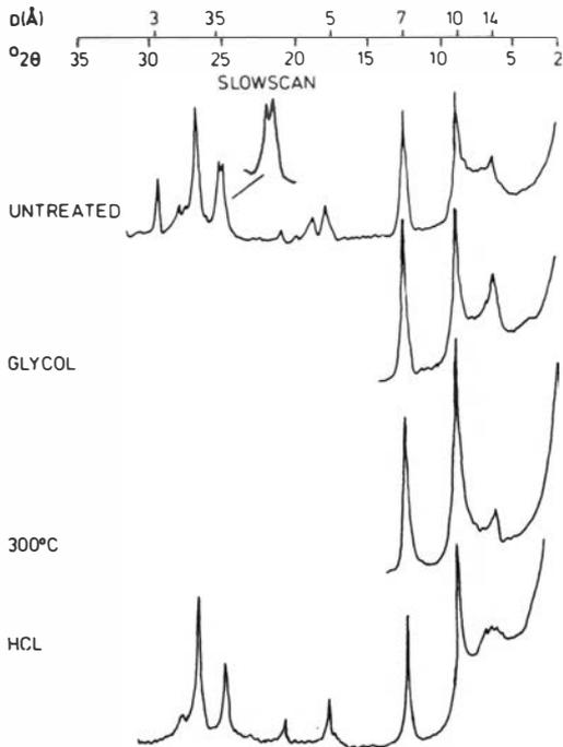
Fig. 7. X-ray diffraction diagrams for the < 2 μm fraction of Quaternary superficial sediments; North Sea, northeastern part. The samples were saturated with Sr<sup>++</sup>.
