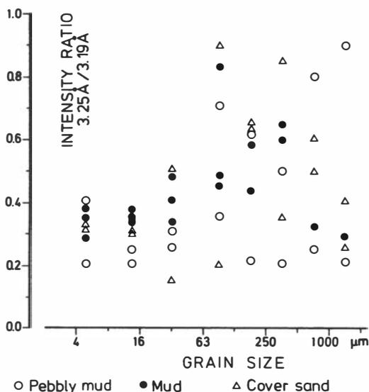
Fig. 12. Plot of the intensity ratio of potashfeldspar and plagioclase in the silt and sand fractions for the different facies.
