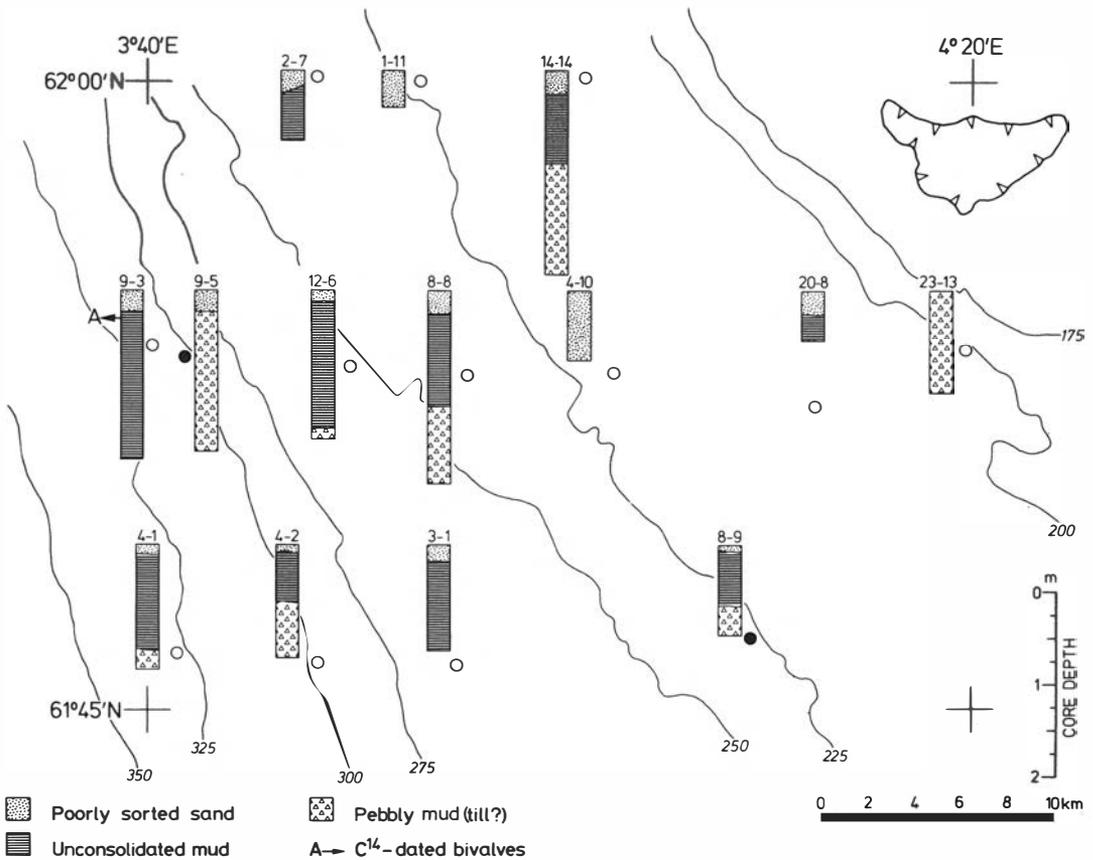
Fig. 2. Bathymetric map showing sample locations and the stratigraphy in the cores. Contour interval: 25 metres. Map is reproduced with permission from Institutt for Kontinentalundersøkelser. Open circle: Samples for detailed sedimentological and mineralogical analysis. Black circle: Samples for stratigraphical analysis.
