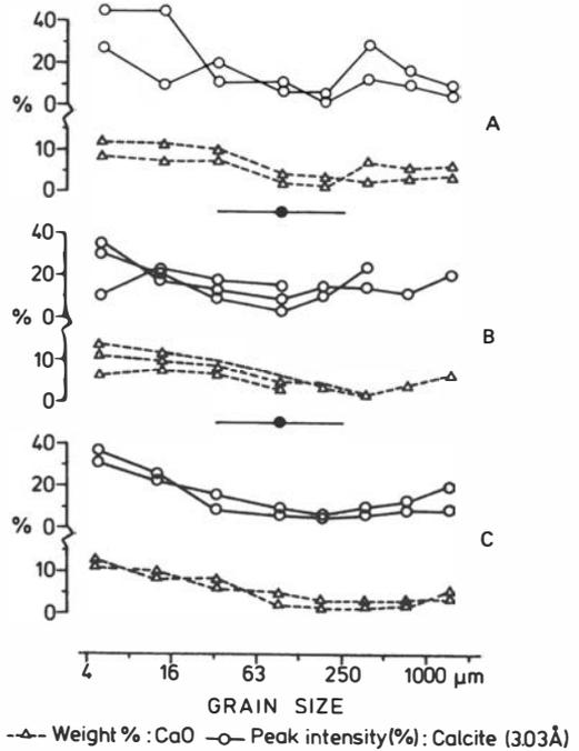
Fig. 10. Plot of the X-ray intensity percentage for calcite and weight % for CaO in the silt and sand fractions for the different facies. (A: Poorly sorted sand, B: Unconsolidated mud. C: Pebbly mud (till?).
