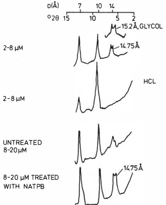
Fig. 6. X-ray diffraction diagram of fine-grained silty sediments after different types of chemical treatments. The samples were saturated with Sr<sup>++</sup>. The natriumtetraphenylborat (NaTPB) treatment extracts potassium from trioctahedral illite, transforming it to a vermiculite mineral at 14.75 Å.
