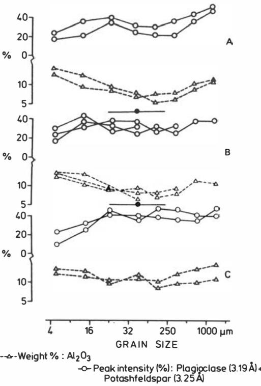
Fig. 9. Plot of the X-ray intensity percentage for plagioclase and potashfeldspar and weight % for Al<sub>2</sub>O<sub>3</sub> in the silt and sand fractions for the different facies. (A: Poorly sorted sand, B: Unconsolidated mud, C: Pebbly mud (till?).
