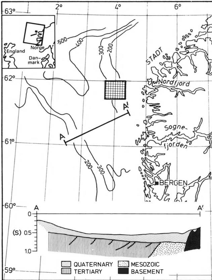
Fig. 1. Location map. The seismic profile (A-A') in two-way reflection time is interpreted as representative for the continental shelf outside west Norway. (A-A'-from Sellevoll & Sundvor 1974).
