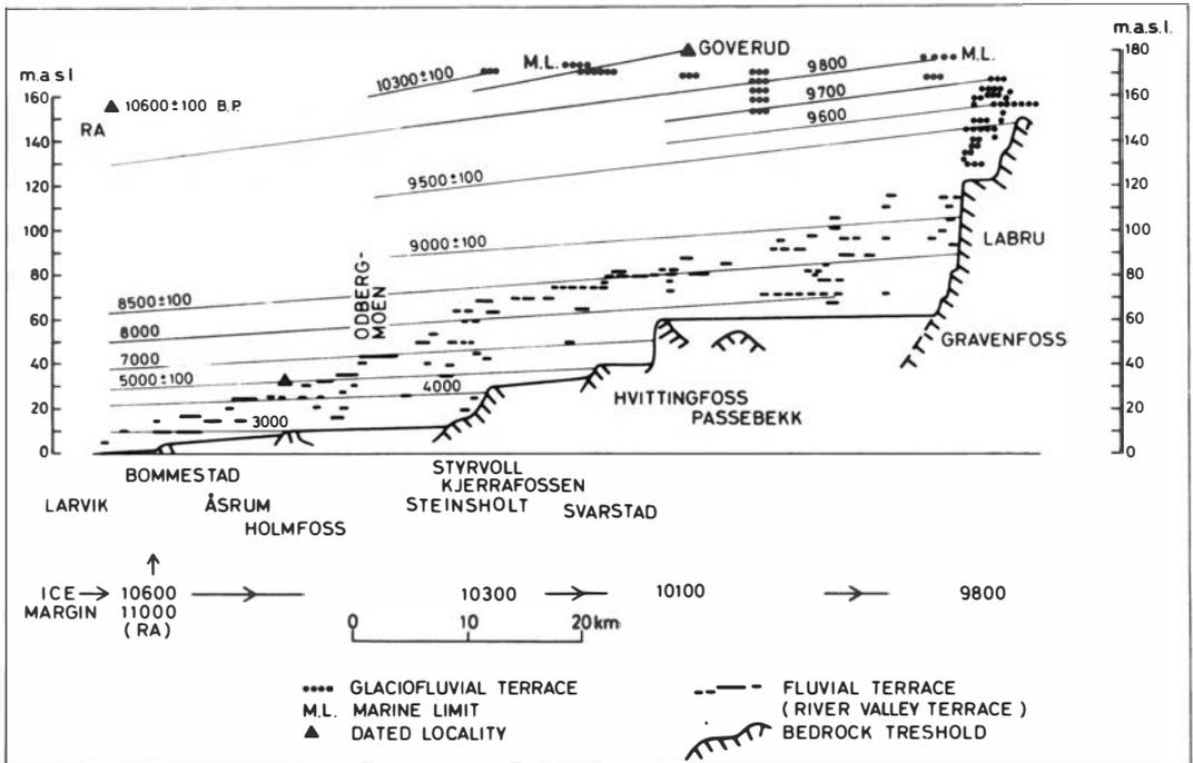
Fig. 2. Profile along the river Lågen from Larvik to Gravenfoss showing bedrock thresholds and elevation of glaciofluvial and fluvial terraces. Equidistant shoreline diagram for the last 10,600 years is superimposed. The profile is parallel to line A-A on Fig. 1.
