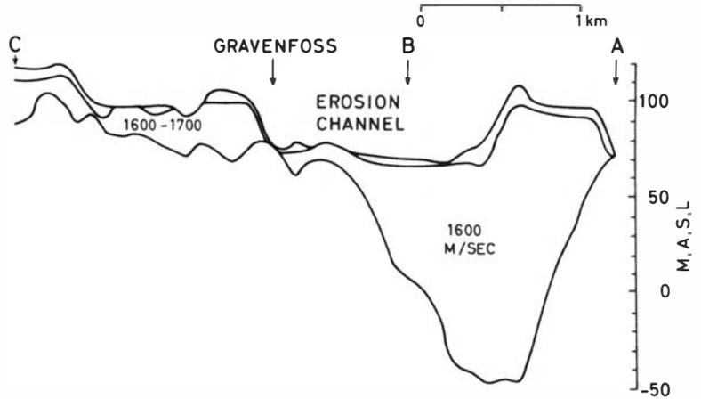
Fig. 4. Depth and seismic velocity of sediments deposited in Numedalfjorden. Seismic profile line A-B-C is shown on Fig. 3. The large erosion channel was probably formed during the Boreal chronozone.
