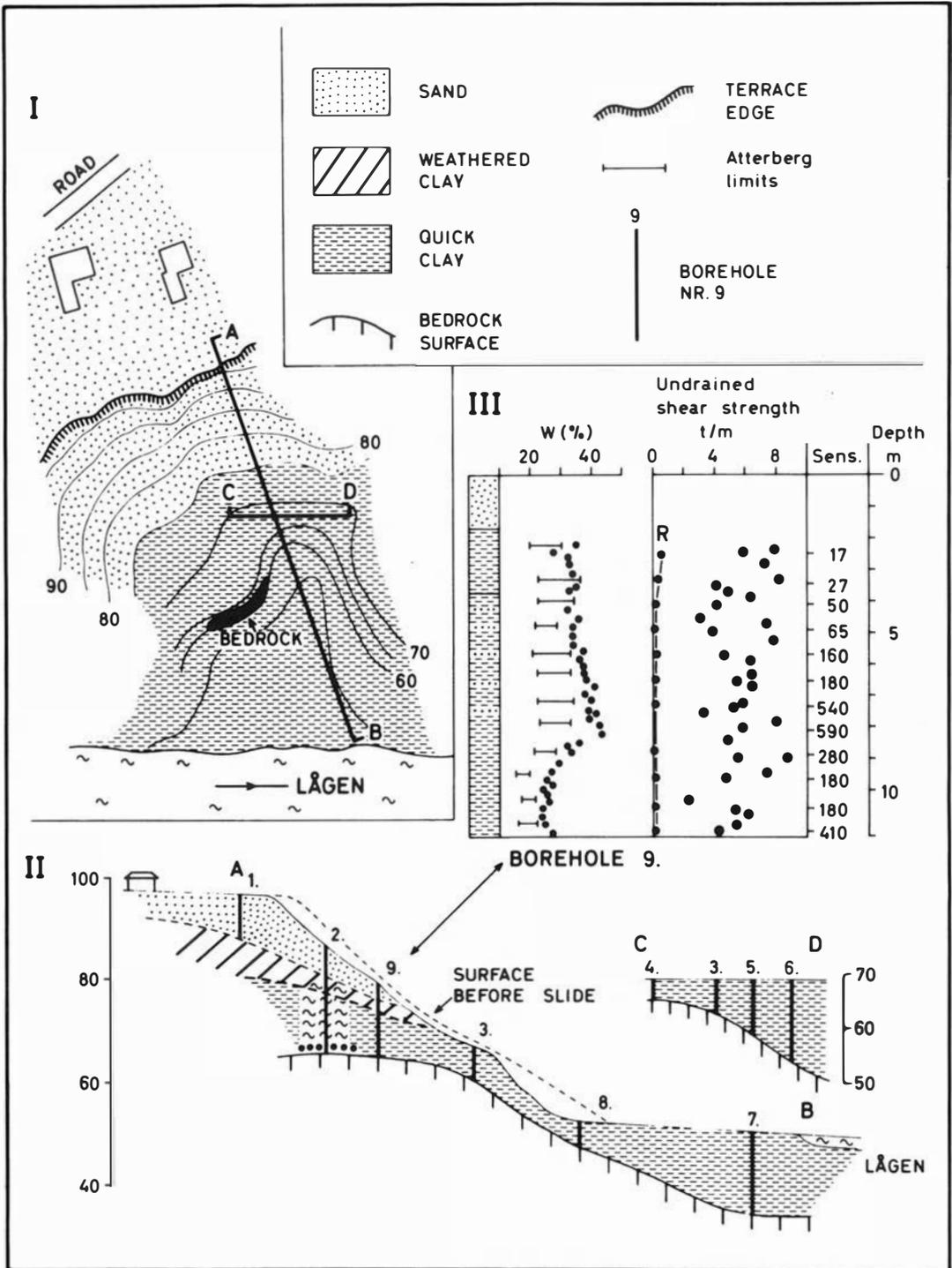
Fig. 6. Section through sediments at Hvitvingfoss. Geotechnical data are from an internal report of Norges geotekniske institutt.
