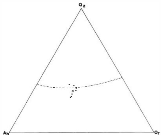
Fig. 1. Plots of ekerite compositions on an orthoclase-albite-quartz ternary diagram. The X represents the average composition of the seven rock samples plotted. Dashed line is the granite cotectic of Tuttle & Bowen (1958) at a water pressure of about 2Kb.
