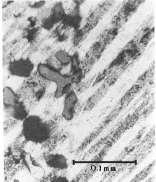
Fig. 3. Photomicrograph of quartz blebs showing some irregular, as well as the more typical spheroidal, shaped blebs. Note also the apparent continuity of perthite lamellae across the blebs.
