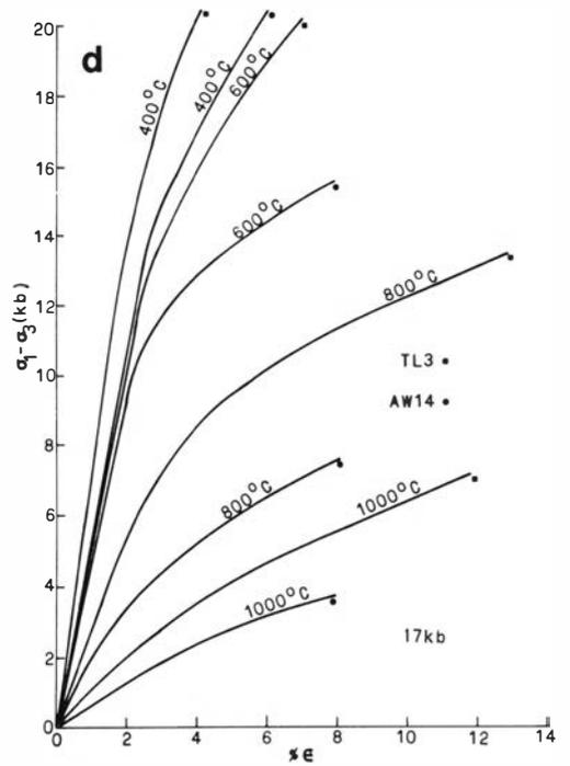
Fig. 2: Stress-strain curves for anorthosite deformed at 400°C to 1000°C and 5 to 17 kb at a constant strain rate of approximately  $10^{-3}$ /second. Each curve is an average of 4 to 10 individual tests. a: Tests at 5 kb, b: Tests at 9 kb, c: Tests at 13 kb, d: Tests at 17 kb.
