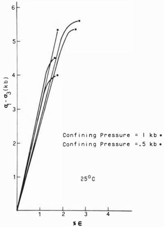
Fig. 1: Stress-strain curves for anorthosite deformed at  $25^{\circ}\text{C}$  and .5 and 1 kb confining pressure. Each curve represents a single test.
