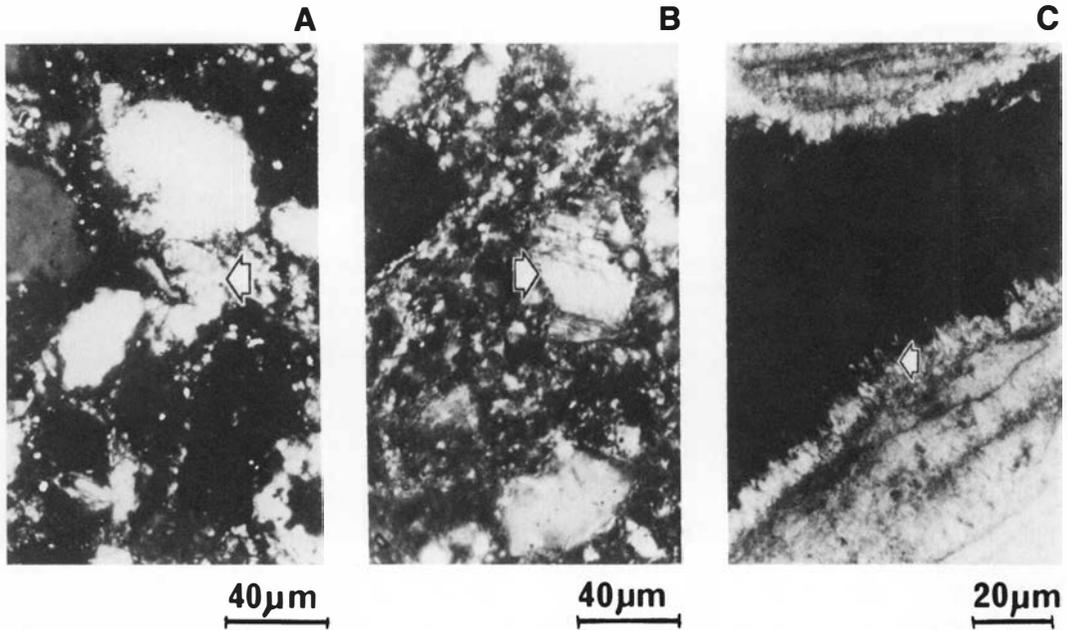
Fig. 1. Thin section micrographs of recent, carbonate cemented sediment from the Sleipner Field, North Sea (A and B) and lithified shallow marine carbonate from Nesøya (C). Arrows indicate cement consisting of low Mg-calcite from the Sleipner Field and high Mg-calcite from Nesøya.
