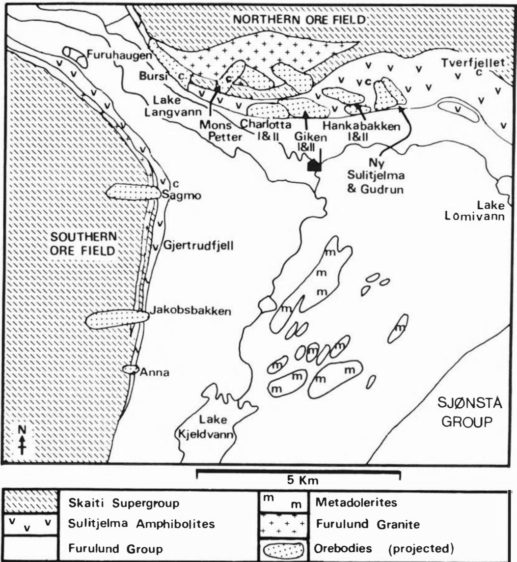
Fig. 1. Simplified geological map of the Sulitjelma area, indicating the main rock units and the location of cotiucles (c).
