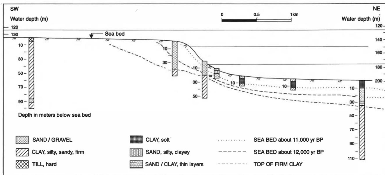
Fig. 2. Schematic section showing the conditions at the edge of the North Sea Plateau (location see Fig. 1). The soil drillings were done for the platform foundation at the Gullfaks Field (after Rokoengen et al. 1982).
