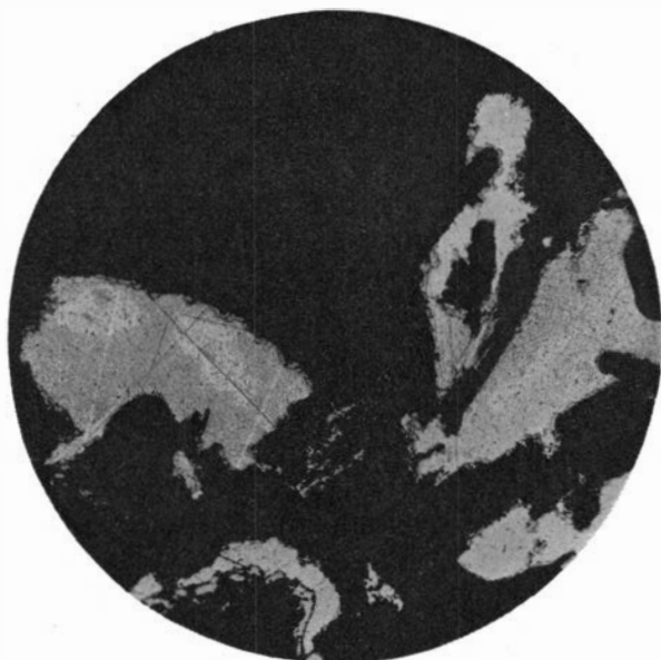
Fig. 4. Quartzite (black) replaced by native copper (grey) and native silver (light grey) within a thin coating of cuprite (dark grey). The borders between copper and silver are smooth, but no crystal faces are seen.
