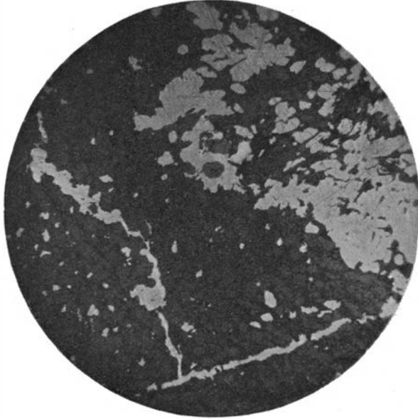
Fig. 3. Native copper (light grey) replacing quartzite (dark grey to black). Smaller portions of native silver (lighter grey) together with native copper.
