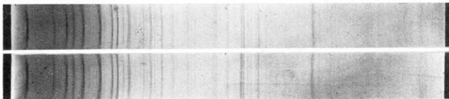
Fig. 2. X-ray powder diagrams of euclase, 9 cm camera, iron radiation with manganese filter. Upper diagram: euclase from Muso, Brazil, lower diagram: euclase separated from beryl pseudomorphs from Hovåsen, Eptevann, Iveland.
