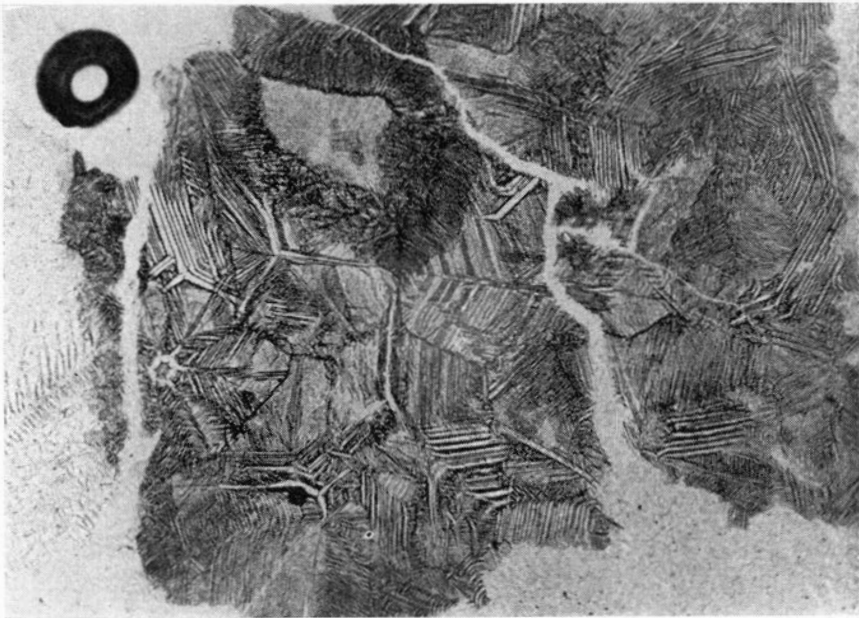
Fig. 3. Nepheline from a corroded refractory stone.
