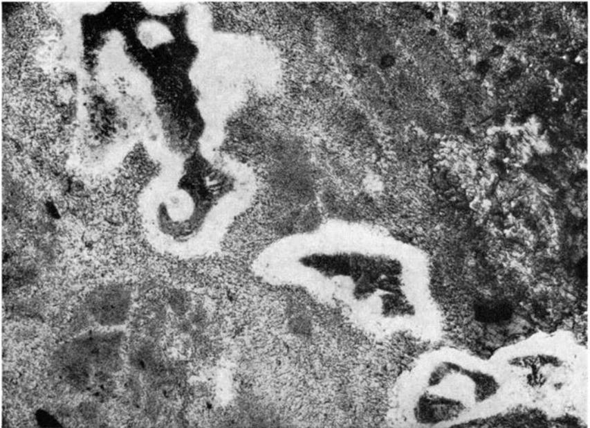
Fig. 2. A corundum-plagioclase kelyphite with rather lobate boundaries due to replacement by plagioclase. The kelyphite is surrounded by a wide zone of recrystallised plagioclase, the main groundmass is a fine grained amphibolite. (locality 6). ( $\times 30$ ).
