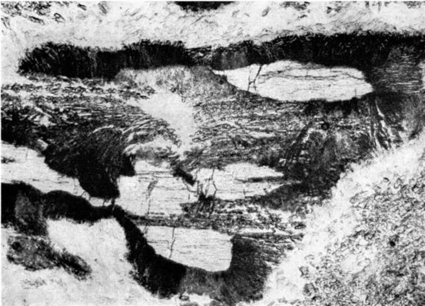
Fig. 2. A large kyanite which shows replacement by a fine, hair-like corundum-plagioclase kelyphite. This kelyphite recrystallises into larger crystals which form transverse aggregates. (locality 7). ( $\times 30$ ).
