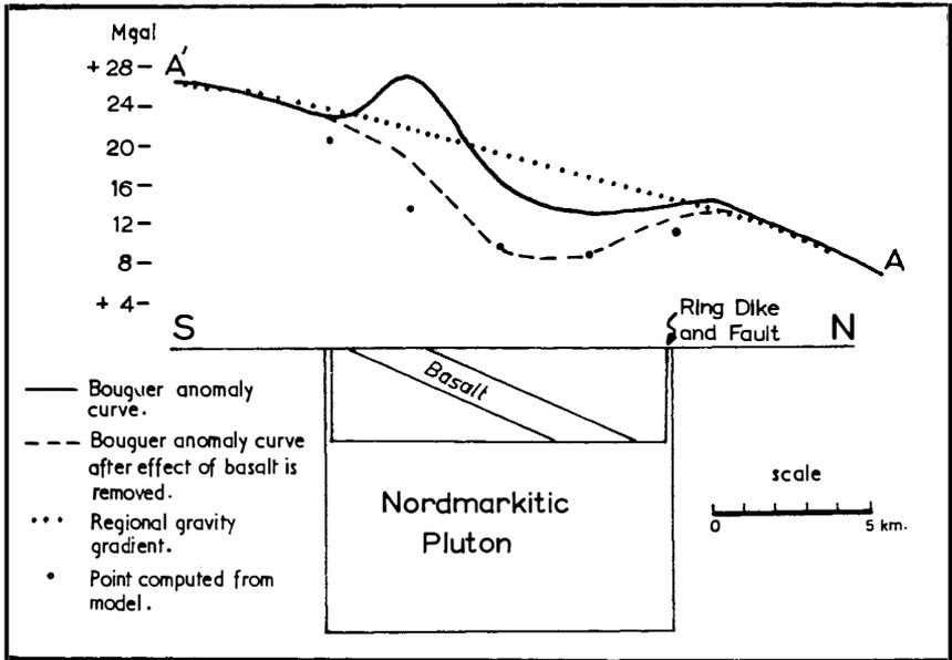
Fig. 3. Profile of gravity field and computed model of nordmarkitic pluton.
