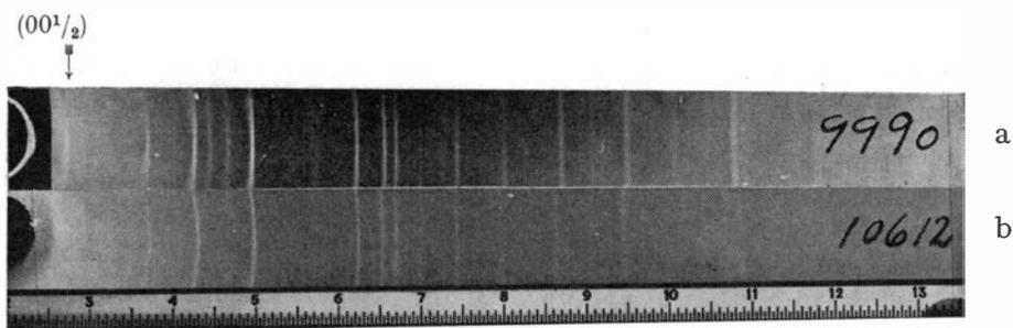
Fig. 2. Reproduction of the X-ray powder patterns. a. Synchisite from Kongsberg. Note the presence of the  $(00\frac{1}{2})$  reflection. X-ray film no. 9990. Geologisk Mineralogisk Museum, University of Oslo. b. Synchisite from Narsarsuk, Greenland.  $(00\frac{1}{2})$  reflection is absent. X-ray film no. 10612. Geologisk Mineralogisk Museum, University of Oslo.
