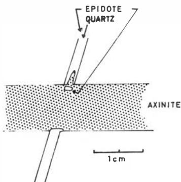
Fig. 6. Oblique intersection of axinite and epidote veins, the latter not being offset by emplacement of the former vein. Relics of epidote occur along the former epidote vein. The epidote vein is axinitized near the intersection. Forbordfjell.
