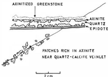
Fig. 7. Replacement origin of axinite veins indicated by oblique intersection with no displacement, gradational border on one side of the vein, and by axinitization of country rock plagioclase along narrow vein. Granmoen, Lökken.
