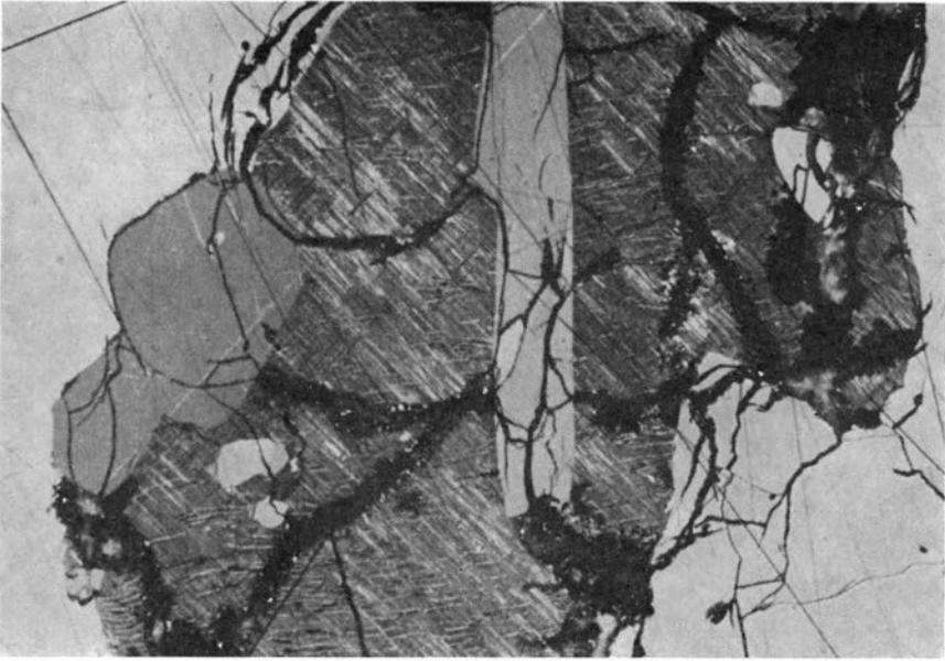
Fig. 2. Magnification  $\times 60$ , oil immersion, + N. The same photo as number one but taken with crossed nicols. The high anisotropism of idaite is very clearly brought out. Also the anisotropism of enargite is very easily visible. The light specks within the thicker cracks are covellite.
