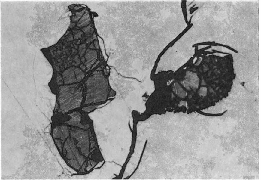
Fig. 3. Magnification  $\times 160$ , oil immersion. Two bornite grains lie within chalcopyrite. The numerous cracks which were called 'fracture disease' are very well developed.
