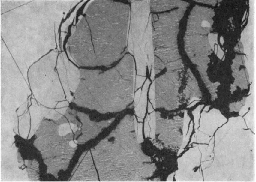
Fig. 1. Magnification  $\times 60$ , oil immersion. Bornite (gray) has spindle-like exsolution lamellae of chalcopyrite and very fine lamellae of idaite; chalcopyrite is white. Two grains (light gray), the one in bornite and the other one bordering bornite and chalcopyrite are enargite. The characteristic cracks are seen very clearly. The thicker cracks are partly filled with limonite and covellite of the 'blaubleibender' type.
