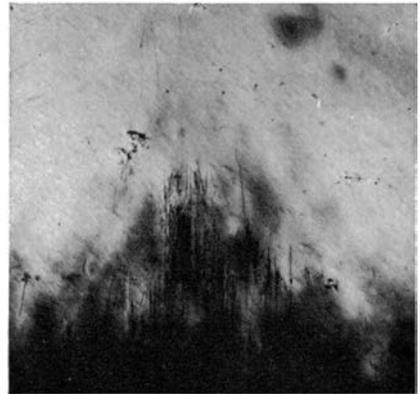
*Fig. 2.* Etch tunnels associated with triangle-shaped Brazil twins. View parallel to the c-axis; in polarized light. Evje, Norway.  $\times 30$ .
