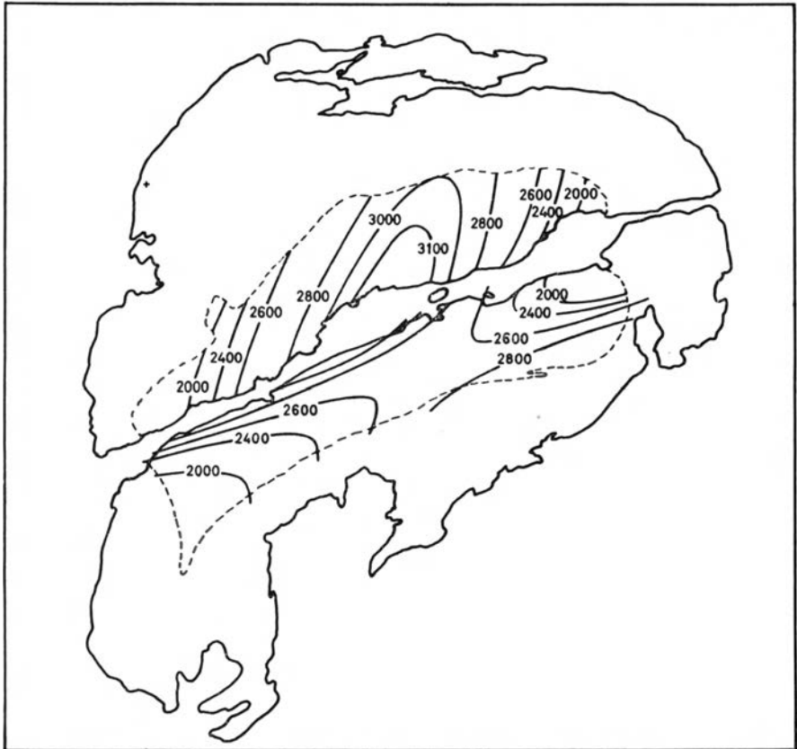
Fig. 4. Fe_{tot} isopleth map of Langø and Gumø. Numbers are counts per second of Fe specific radiation. Map based on separate calculations for each of the islands displays excellent agreement of contours. 2nd degree polynomial.
