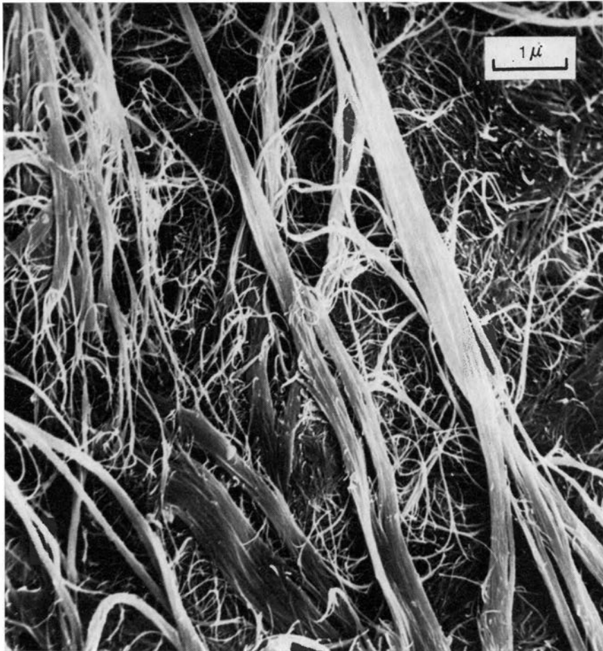
Fig. 2. Scanning electron micrograph of a flake of mountain leather. A tendency for a preferred orientation of the broader aggregates of fibrous crystals is shown. The flexible nature of the thinner palygorskite crystals is displayed by their curvature where they are split away from the larger aggregates, probably as a result of the detachment of the flake from the mass of the specimen.
