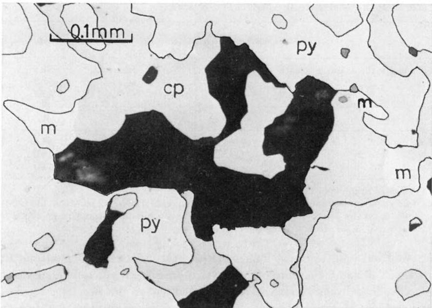
Fig. 2. Ore from Middavarre showing melonite (white, m) in close contact with pyrite (light grey, py). Chalcopyrite (darker grey, cp) and gangue minerals (dark) fill in between the subhedral pyrite grains. Plane polarised reflected light, air, 240 $\times$ .
