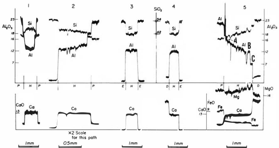
Fig. 2. Composition profiles along the paths shown in Fig. 1. P: pyrope, D: diopside, E: enstatite, H: hornblende.
