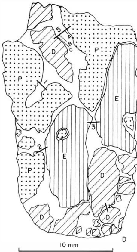
Fig. 1. A diagram of the thin section. The numbered lines shows the paths of electron microprobe analysis. P: pyrope, D: diopside, E: enstatite.
