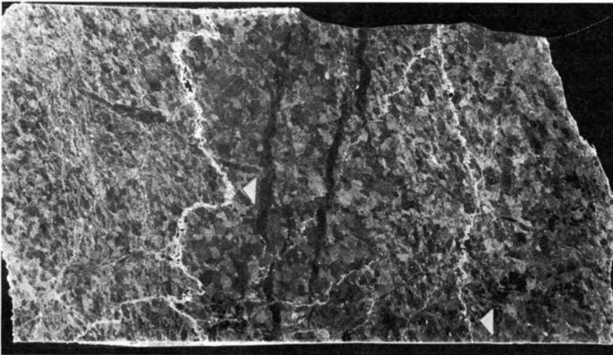
Fig. 2. Peel print from the stylolitic Jøvikelva marble. Arrows mark stylolite seams.
