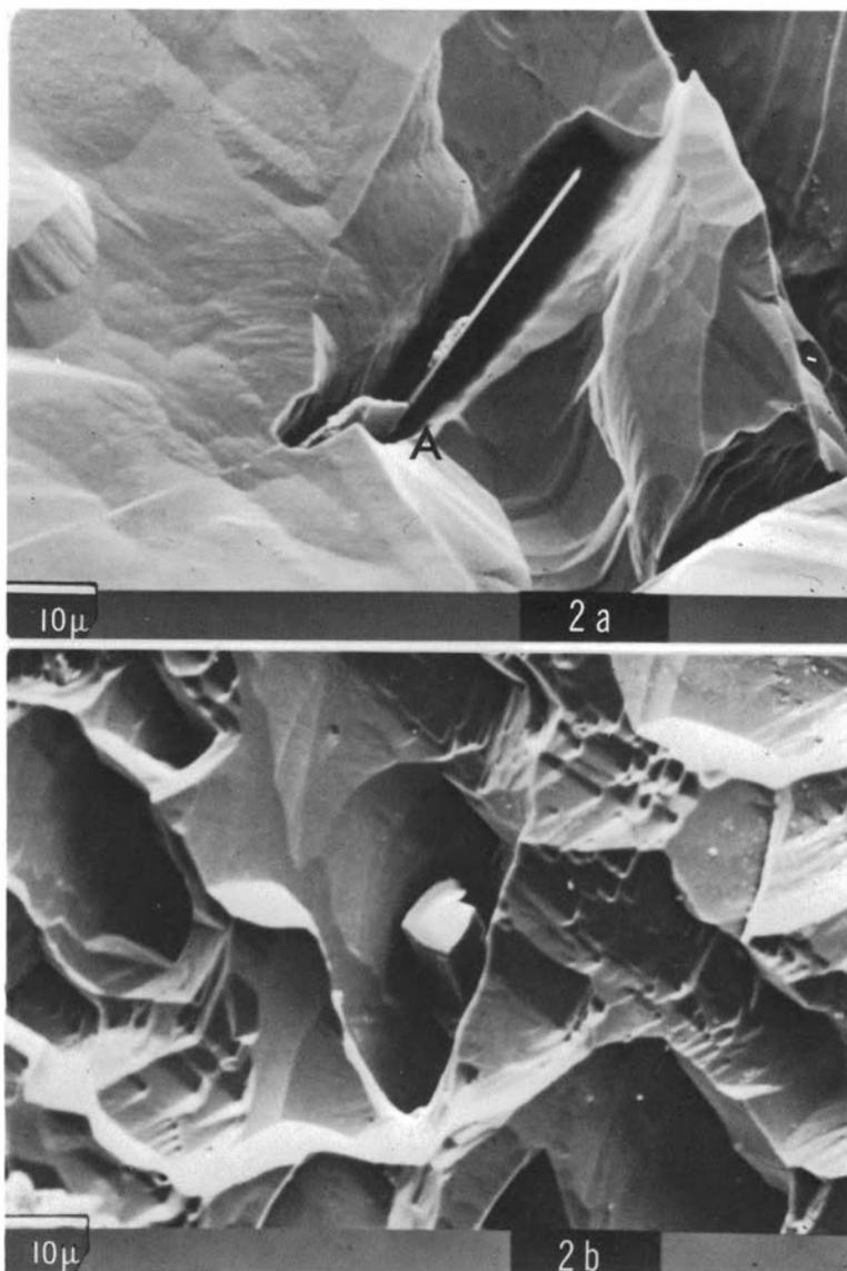
*Fig. 2a.*  $An_{25}$  from Arendal. Two platelets (approximately 0.4 microns in thickness) on different habit planes, giving the appearance of a 'bent' inclusion (at A).
