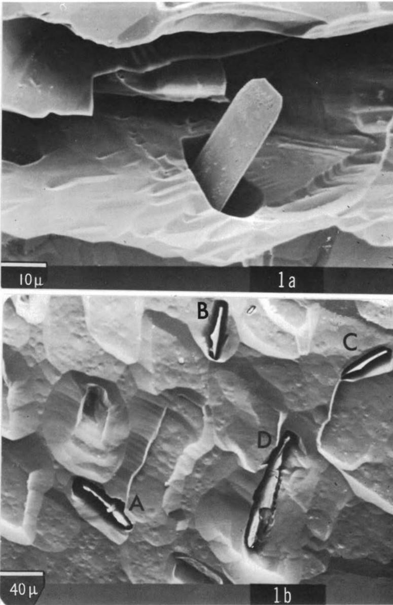
*Fig. 1a.*  $An_{25}$  from Bamle. A typical euhedral hematite platelet in a feldspar matrix. (The micron scale on the left of this and all other figures refers to the black bar).
