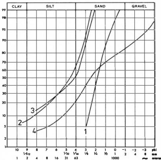
Fig. 5. Grain size distribution curves. Sample 1: Glaciomarine sand. Sample 2: Glaciomarine silt. Sample 3: Massive silt. Sample 4: Till.
