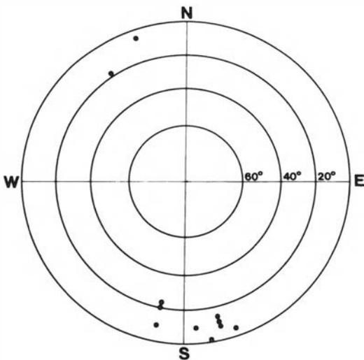
Fig. 7. Fold axes orientation below the discordance, displayed on Schmidt's net (lower hemisphere).
