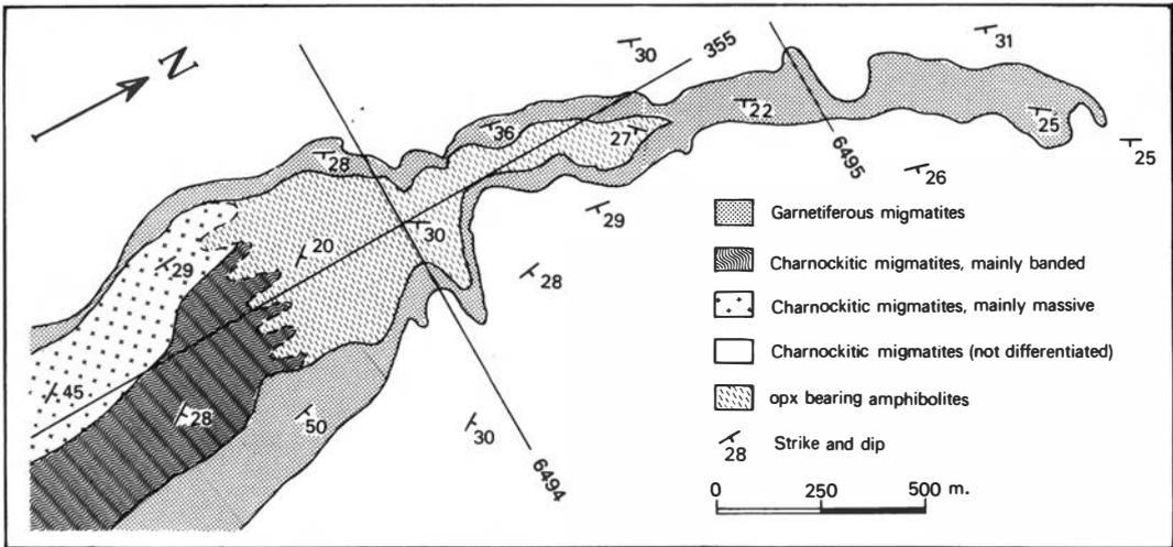
Fig. 3. Map of area around domain L showing the foliation of charnockitic migmatites and amphibolites oblique to lithological boundaries.
