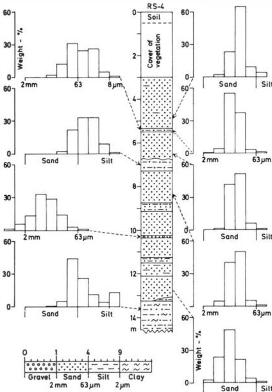
Fig. 8. Grain-size distribution in a section through postglacial fluvial sediments at locality RS-4 (Fig. 1).
