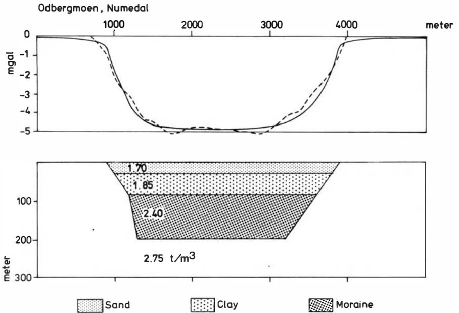
Fig. 7. Residual gravity profile and suggested sedimentary interpretation, based on gravity data.
