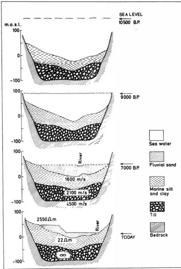
Fig. 10. Suggested stages in the glacial and postglacial development of the area studied. The profile chosen is shown on Fig. 1 by the line C-C. Seismic velocities and VES resistivities are given.
