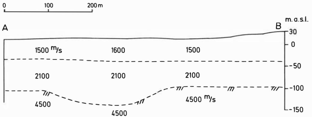
Fig. 3. Results from seismic refraction studies. Profile line A–B is shown on Fig. 1.
