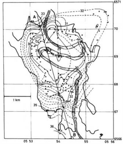
Fig. 6. Bouguer anomaly map (UTM coordinates). Present position of river Lågen shown with horizontal lines. Contour interval 0.5 mgal.
