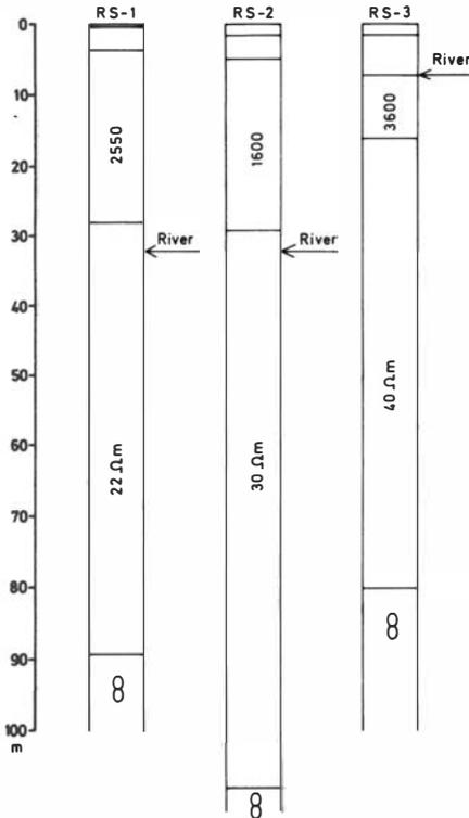
Fig. 5. Results from three vertical electrical soundings. Location on Fig. 1.
