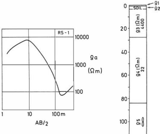
Fig. 4. Field data and interpretation of the vertical electrical sounding (VES) at locality RS-1 (Fig. 1).
