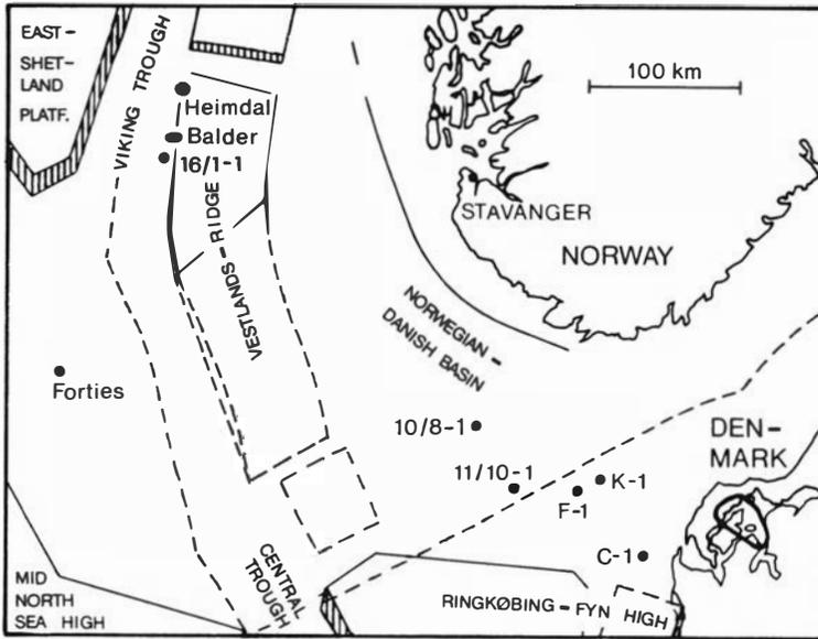
Fig. 1. Map of the North Sea with localities, well-sites, and structures mentioned in the text. (Egelund, based on maps in Bergsager (1980) and Rasmussen (1974, 1978)). Approximate extent of the 'Mo-clay area' indicated in North Jutland. The late Palaeocene shore line probably was not far from the present west coast of Norway and was bending along the Fenno-Scanian border-zone through the northern tip of Jutland (cf. Bonde 1973, 1979).
