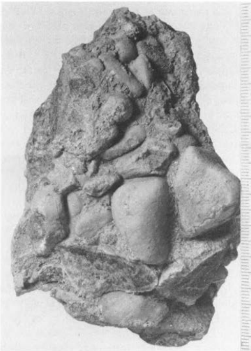
Fig. 4. Hand-specimen taken from part of the central pebbly zone of the breccia, showing the rounded nature of the abraded fragments and their zeolite crust. Scale in mm and cm.
