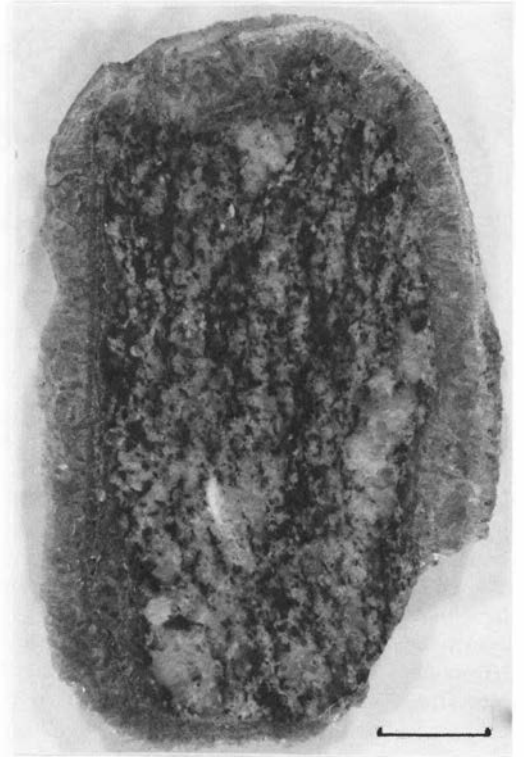
Fig. 5. Photograph of a sliced 'pebble' of abraded granite gneiss showing the radiate stilbite encrustation. The very outermost 0.5–1 mm rind is composed of a creamy white aggregate of microcrystalline quartz and some stilbite. Bar = 1 cm.
