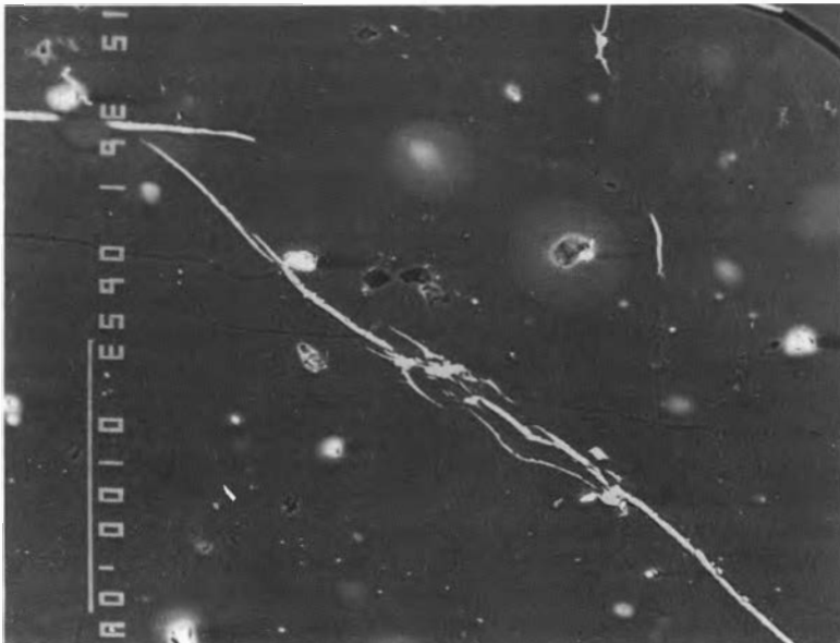
Fig. 4. Back-scatter electron micrograph of Nb-Ta minerals filling veins and fractures in the hydrocarbon (scale bar 100 \mu\text{m} ).
